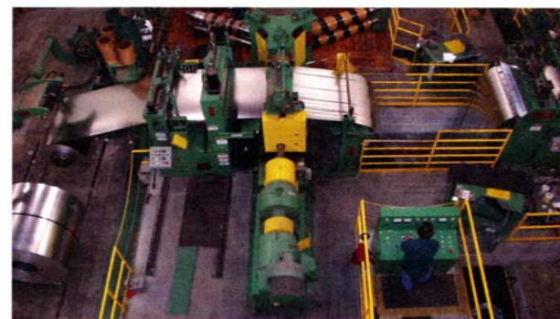
Calstrip's 60-inch triple-head Braner USA slitting line located at the company's Southwest Steel Coil plant in New Mexico.
