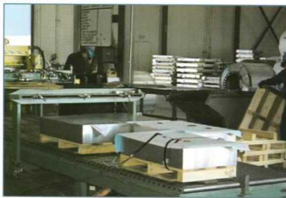
Blanks ready for packaging and shipment, cut from a parent coil
